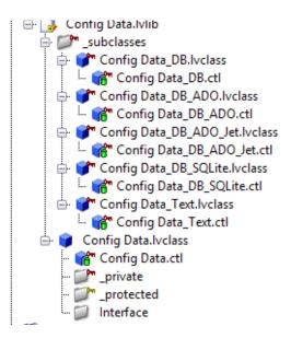
For a class hierarchy, the framing consists of the class files and the directory structure to hold them. As explained before, I create a directory structure in the class' base directory that mirrors this structure. Note that I have also created some virtual folders inside the *Config Data* class which represents actual subdirectories.
