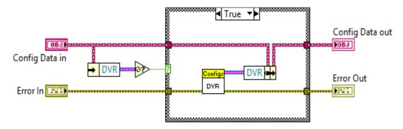
If the DVR in the class data is not valid, I call the DVR VI to get a valid reference and then use that reference to populate the class data. If the DVR reference is valid, the false case does nothing but pass on the class data unmodified. When I save this VI, I put it in a subdirectory named *\_protected*.
